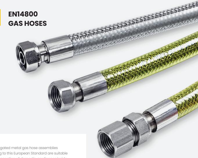
The corrugated metal gas hose assemblies according to this European Standard are suitable for the connection of domestic appliances inside or outside a dwelling using gas at a pressure lower than 0,5 bar. Gas hoses are suitable for 1st, 2nd and 3rd family gases. These gases are commonly refered to as manufactured gases, natural gases and liquid petrolium gases (LPG).
