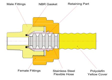
Paktermo Safe Assemble System provides long-lasting and safe use due to its components.
